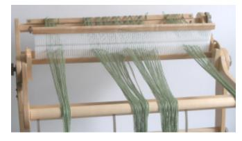
To add in the pre-wound dyed sections, hold the pre-dyed warp chain at the cross with your fingers holding the cross open. Pull each loop through the slots of the reed in order. Slip them onto the back warp beam stick if you can, or tie them in small bundles to the beam. After the chains are attached firmly to the warp beam be sure to adjust the dyed warp chains by gently pulling the entire warp bundle at the choke tie (the one past the cross). This will help keep the threads in the dyed stripe
