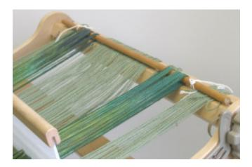
Use whatever method you like for spreading the warp. We usually weave about 1½" of waste yarn at the beginning and again at the end of the fabric. Weave the entire length of the warp using the solid color of Dragon Tale cotton. For two 28" towels, or one 58" runner, you will need to weave 66" of fabric measured with the tension released.
